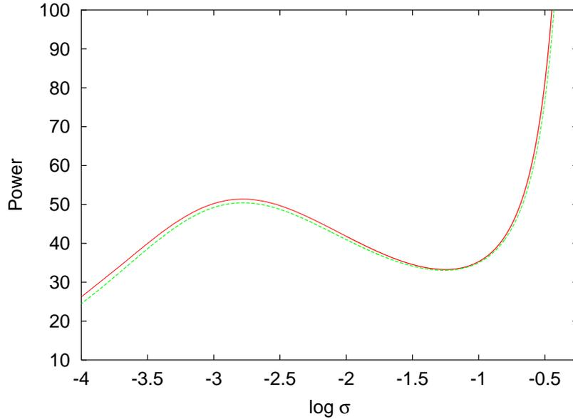
Figure 1: The power versus propagation constant ( $P$  versus  $\log \sigma$ ) curve for the 1-D colloidal solitary wave. Shown are the semi-analytical (solid lines, red) and numerical (dashed lines, green) solutions. The background fraction is  $\eta_0 = 1 \times 10^{-3}$ .
