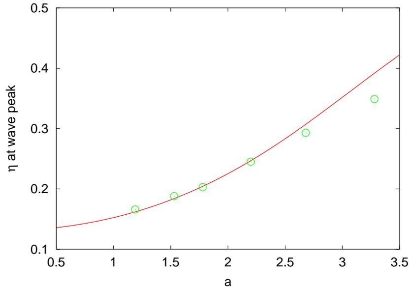
Figure 7: The neutral stability curve in the amplitude-maximum packing fraction plane ( $a, \eta$ ) for the 2-D colloidal solitary wave. Shown is the semi-analytical solution (solid line, red) and numerical solutions (circles, green).
