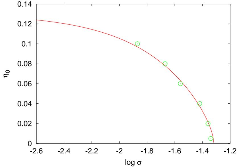
Figure 6: The neutral stability curve in the propagation constant-background packing fraction plane ( $\log \sigma$ ,  $\eta_0$ ) for the 2-D colloidal solitary wave. Shown is the semi-analytical solution (solid line, red) and numerical solutions (circles, green).
