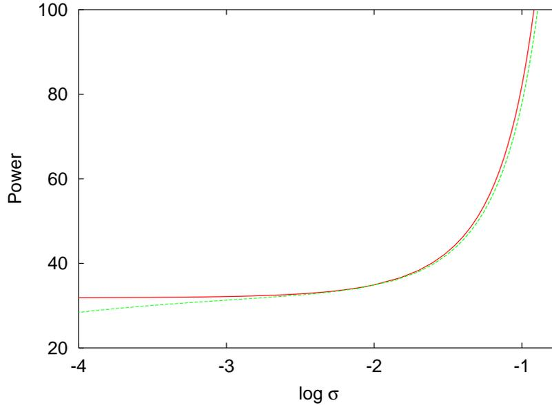
Figure 5: The power versus propagation constant ( $P$  versus  $\log \sigma$ ) curve for the 2-D colloidal solitary wave. Shown are the semi-analytical (solid lines, red) and numerical (dashed lines, green) solutions. The background fraction is  $\eta_0 = 0.3$ .
