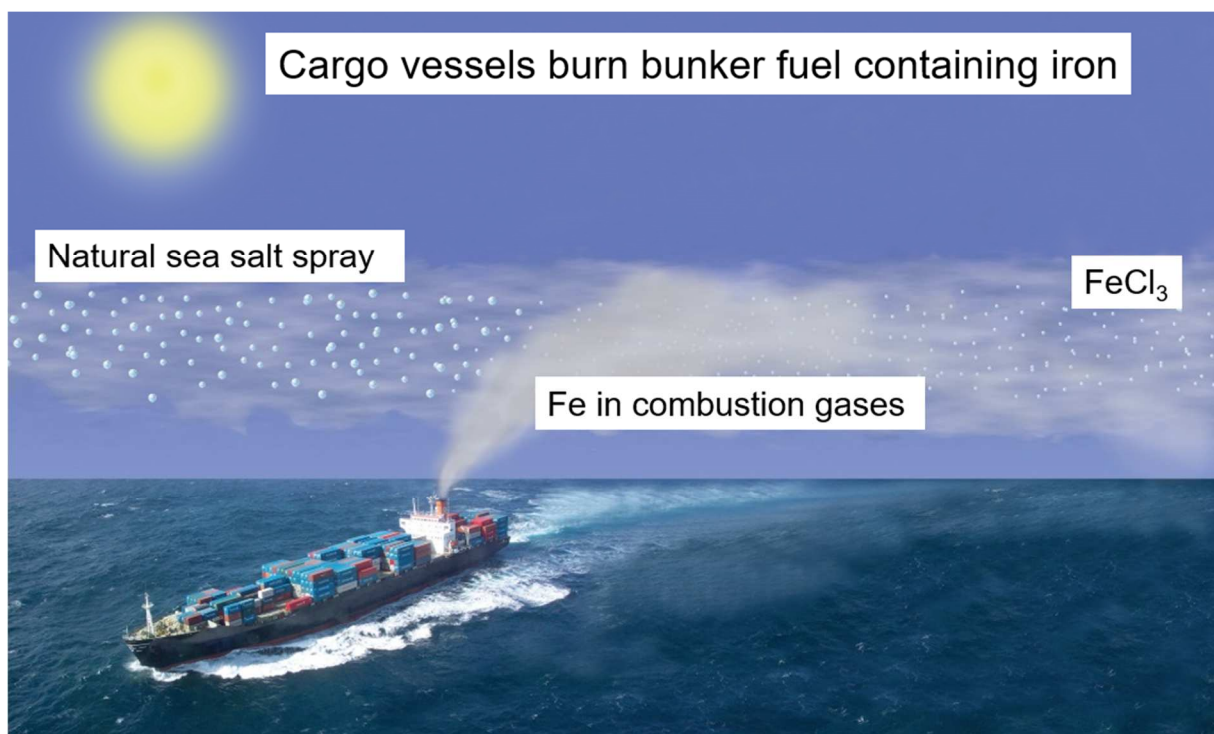
Figure 2: A container ship powered by bunker fuel mixed with commercially available iron additives [73, 74] which are sold to reduce black carbon and carbon monoxide (CO) emissions and to reduce fuel consumption. In the exhaust plume, the iron compounds react with sea salt to produce iron chloride (FeCl 3 ), which under sunlight generates Cl atoms [69] that oxidize CH 4 16 times faster than °OH radicals [71].
