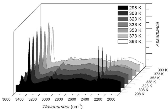
**Figure 2.** Series of spectra taken from an isobar from a single site of a single  $\text{Sc}_2(\text{BDC-NH}_2)_3$  crystal. As temperature increases the magnitude of the adsorbed  $\text{CO}_2$  asymmetric stretch at  $2335\text{ cm}^{-1}$  wavenumbers decreases relative to the  $\text{NH}_2$  symmetric and asymmetric stretches.
