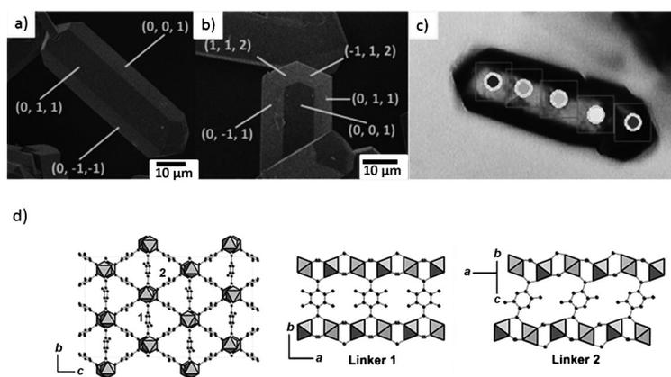
**Figure 1.** a,b) SEM of  $\text{Sc}_2(\text{BDC-NH}_2)_3$  crystals with face indices marked ( $10\ \mu\text{m}$  scale bars shown), c) optical micrograph showing sites selected on the same crystal for IR analysis, (boxes represent  $10 \times 10\ \mu\text{m}$  area from which spectra are collected). d) Framework structure of  $\text{Sc}_2(\text{BDC-NH}_2)_3$  ( $\text{ScO}_6$  gray octahedra, C and N atoms shown as spheres (all possible N atom positions included and H omitted).
