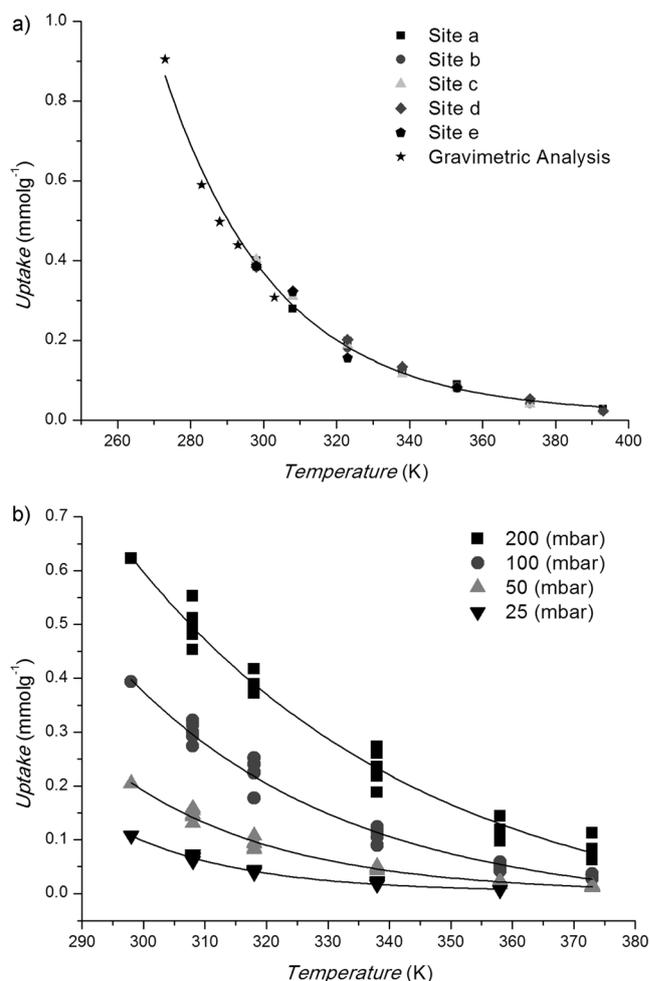
**Figure 3.** a)  $\text{CO}_2$  isobar ( $P_{\text{CO}_2} = 0.1\text{ bar}$ ), measured on 5 sites (Figure 1c) on a single crystal at 298–393 K (square, site a; circle, b; triangle, c; diamond, d; pentagon, e). Comparison between uptakes from single crystal IR data and conventional gravimetric adsorption (stars), fitted by an exponential curve calculated assuming a heat of adsorption of  $31\text{ kJ mol}^{-1}$ . b)  $\text{CO}_2$  isobars ( $P_{\text{CO}_2} = 25, 50, 100, 200\text{ mbar}$ ).
