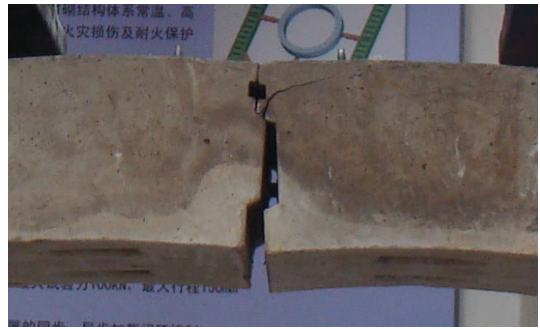
(c) Joint bolts yielding (RCJ2)
