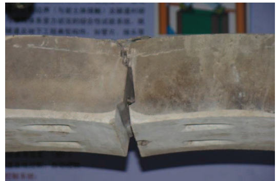
(e) Joint bolts yielding (RCJ3)
