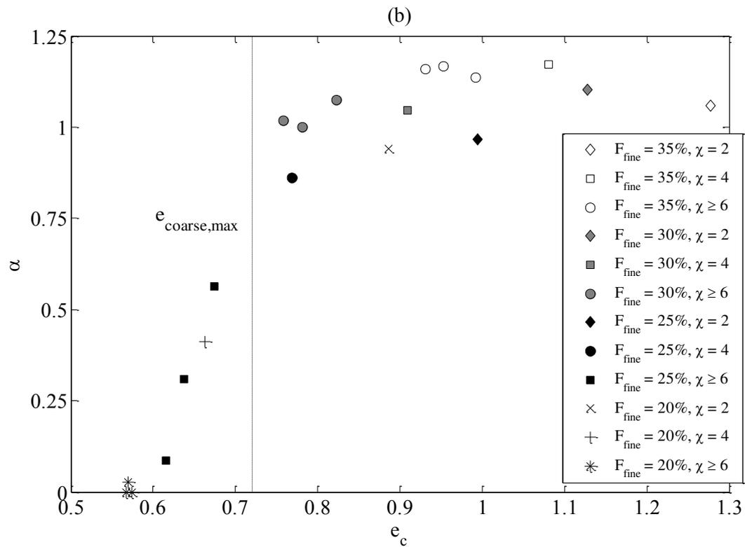
Figure 8. Variation of stress-reduction  $\alpha$  with (a) coarse-coarse coordination number; (b) coarse void ratio.  $e_{\text{coarse,max}}$  value for monodisperse glass beads taken from Cho et al. (2006).
