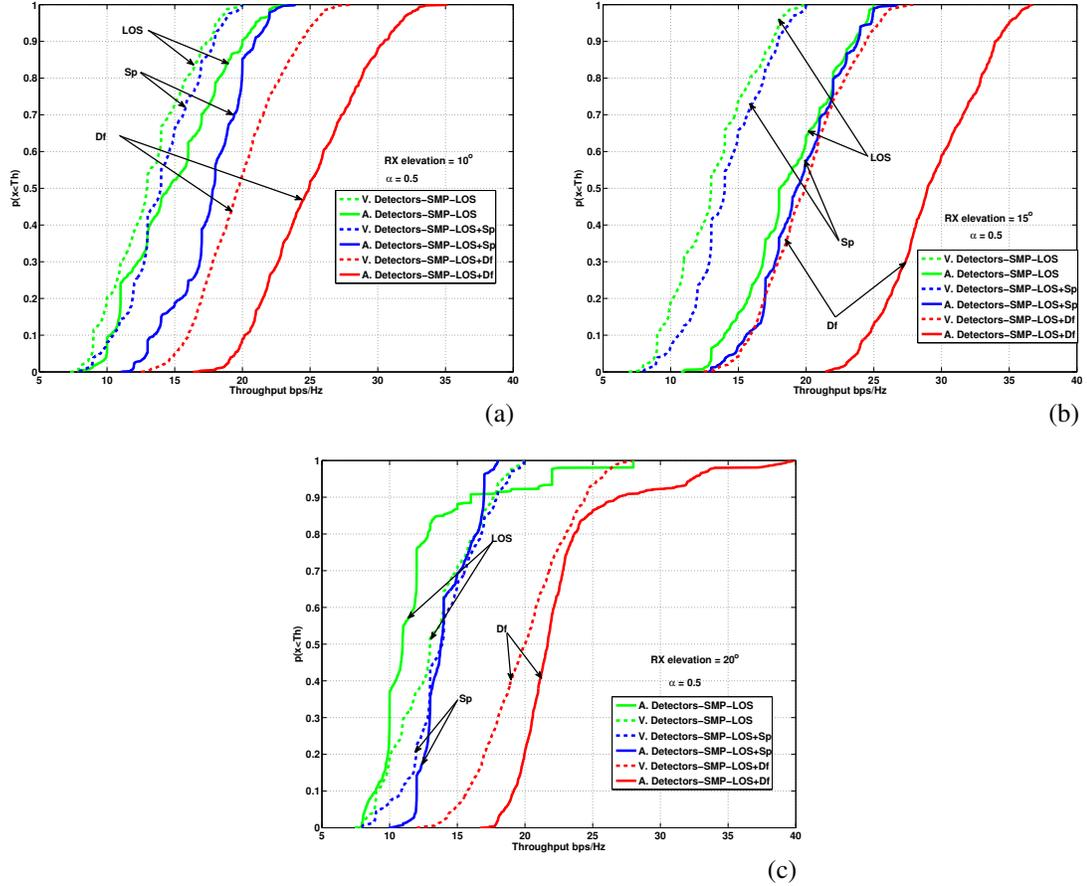
Fig. 5. SMP CDF comparison between three elevation angles in angular diversity receiver detectors when LOS, LOS + Df and LOS + Sp are considered,  $\alpha = 0.5$  (a) SMP,  $10^\circ$  (b) SMP,  $15^\circ$  (c) SMP,  $20^\circ$
