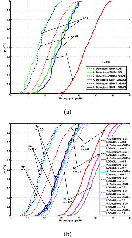
Fig. 9. SMP CDF comparison between three reflection coefficients in vertically and angular diversity receiver detectors when LOS, LOS + Sp and LOS + Df are considered (a) LOS Vs LOS + Sp,  $\alpha = 0.3$  (b) LOS + Sp Vs LOS + Df comparison,  $\alpha = 0.3, 0.5$  and  $0.7$ .
