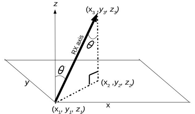
Fig. 2. Geometry for elevation angle calculations
