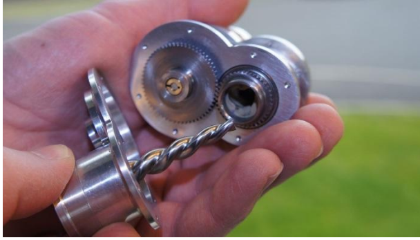
Figure 10. Hermetic assembly cooler based on the MK03 compressor
