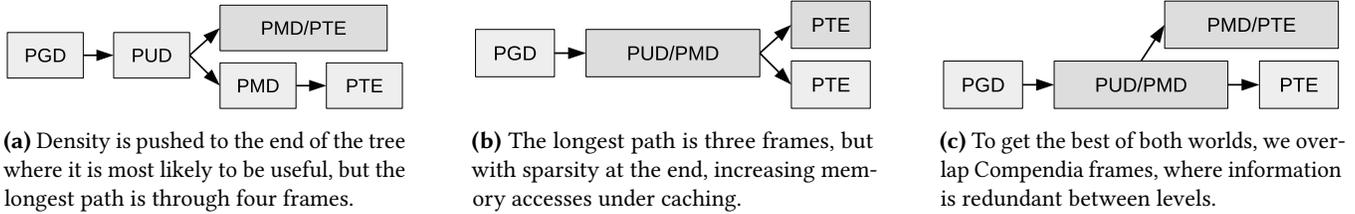
**Figure 9.** With different density patterns down each path, there is a conflict over the best pattern for each branch. In this example, we assume that the top PMD/PTE level in each diagram is sufficiently occupied to be dense, but the bottom one is not.
