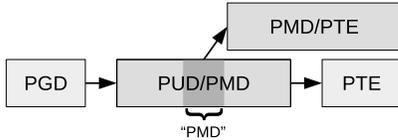
**Figure 10.** Instead of storing 512 different offsets into a Compendia frame within the previous level under overlap, we store 512 copies of the base, each carrying the ‘O’ bit to indicate the need to index with the previous 9 bits as well as the next. This adds the base of the entire PMD/PTE frame to the cache for next time, avoiding PUD/PMD lookup.
