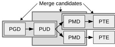
**Figure 8.** When multiple levels feature the requisite level of density, then we are faced with a choice in how to densify the merged radix-tree levels. Typically, it is best to merge closer to the PTE, as the number of entries increases exponentially down the hierarchy, and thus entries become less cacheable.
