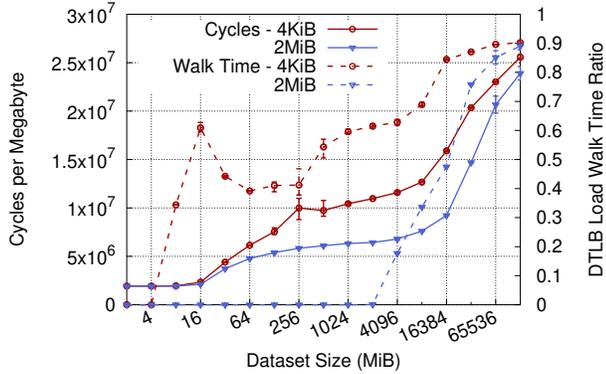
**Figure 5.** CPU cycles of execution time per megabyte of data input (left), and fraction of cycles with active page-table walks (right), on RandomAccess, with increasing dataset sizes for 4 KiB and 2 MiB pages. If execution time increased proportionately with input size, *Cycles per Megabyte* would be flat. When spikes in *DTLB Load Walk Time Ratio* correlate with *Cycles per Megabyte*, an extra layer of page-table-walker cache misses (PGD→PUD→PMD) occurs.
