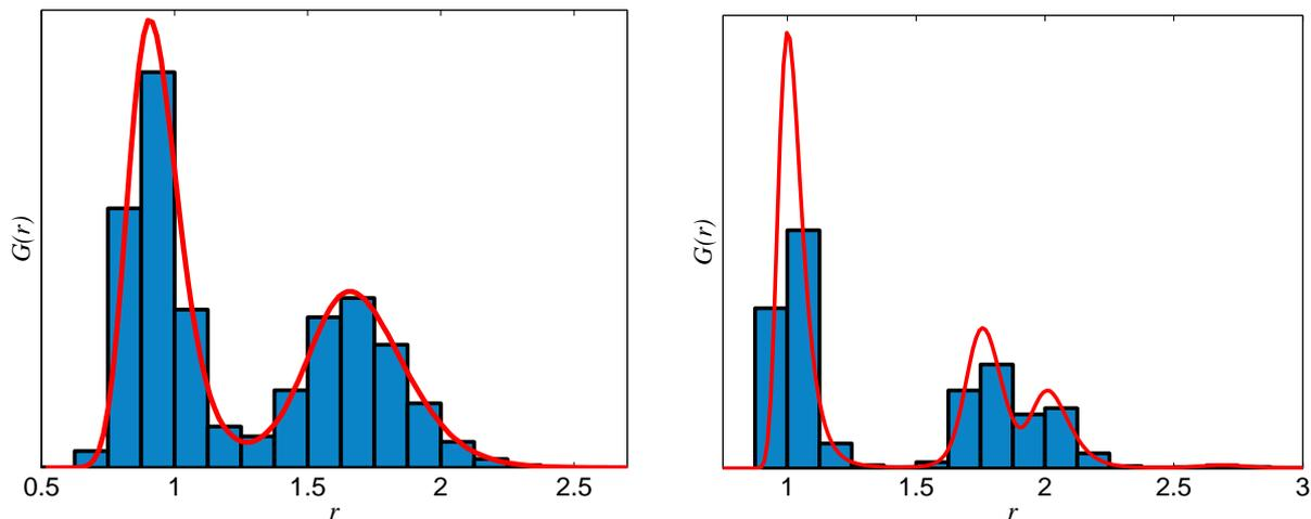
Figure 3: The diagrams illustrate the distributions of interatomic distances,  $G(r)$ , for Morse (left) and Lennard-Jones (right) clusters. They also show the choice of bins used in calculating the numerical distributions.
