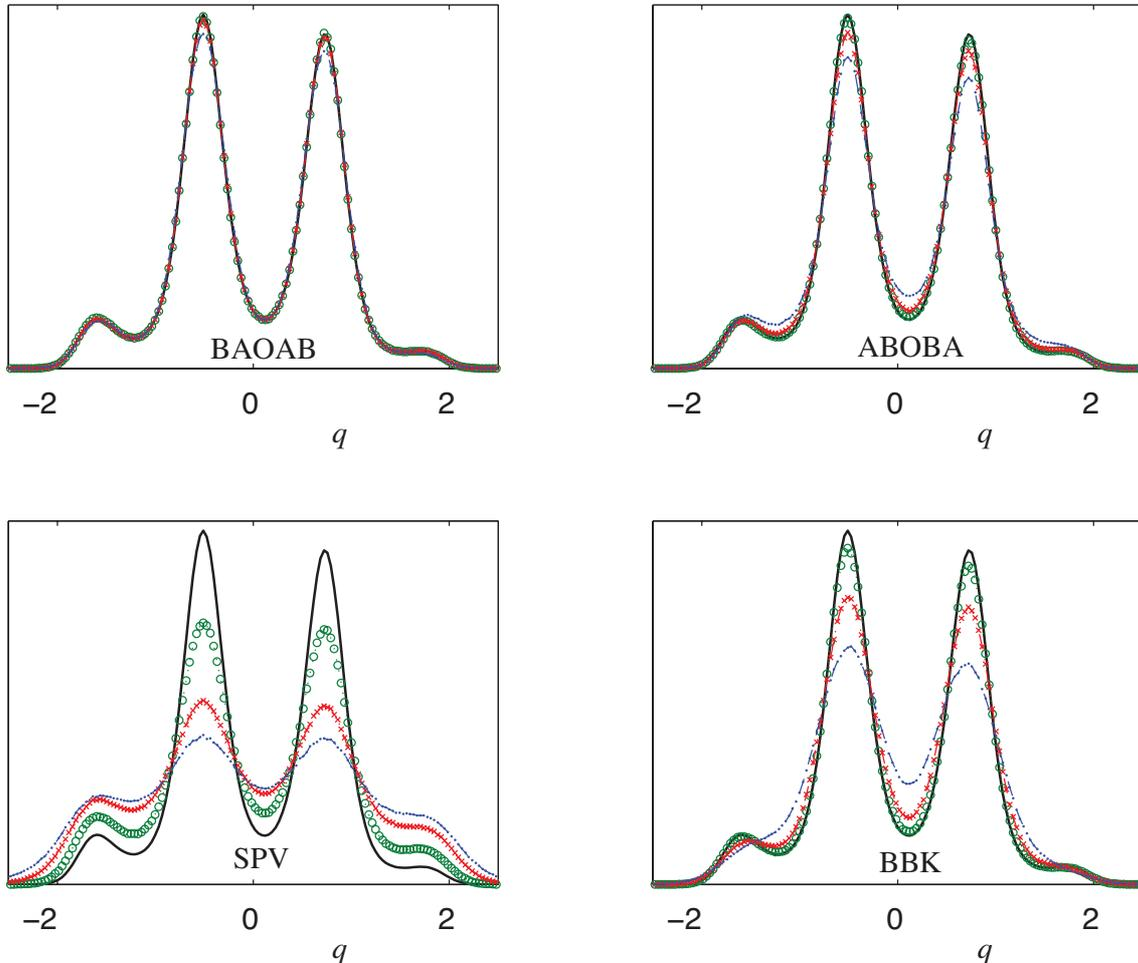
Figure 2: Computed distributions of the 1D model problem are compared for  $\gamma = 20$ . The three curves for each of the four methods show the results for three different stepsizes:  $\delta t = 0.1$  (circles),  $\delta t = 0.2$  (crosses),  $\delta t = 0.3$  (dashed), compared to the dark, solid curve representing the exact distribution. The graph shows that the generalized GLA methods are superior to SPV and BBK in the moderate  $\gamma$  regime.
