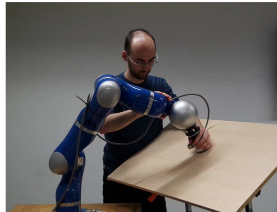
Fig. 9. Demonstration of a circular wiping trajectory on a flat surface. The demonstration was repeated on 12 surfaces of different orientations.
