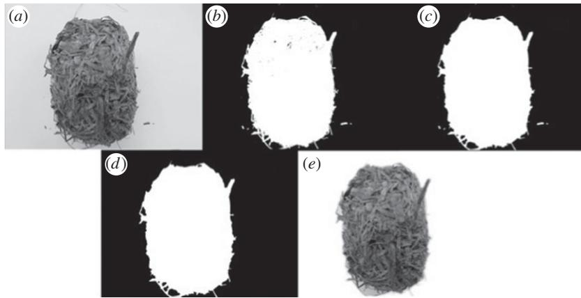
**Figure 2.** Image processing steps to remove small objects and background. (a) Original image; (b) binary image; (c) image after closing operation; (d) removing of all connected components from the binary image associated to noise; and (e) original image without noise and background.
