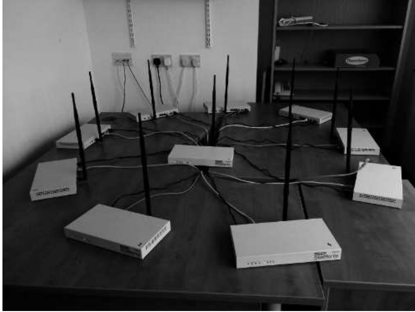
Figure 4: Test bed used for the evaluation of the proposed proportional-fair allocation scheme. We use nine Soekris net6501-70 devices, one acting as AP and the others as stations.
