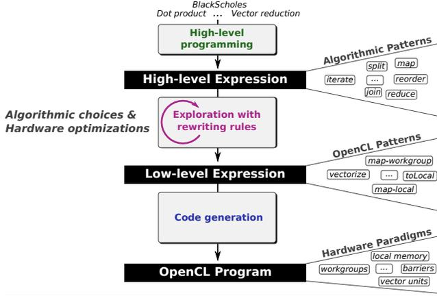
**Figure 1:** Overview of our system. The programmer expresses the problem with high-level algorithmic patterns. These are systematically transformed into low-level OpenCL patterns using a rule rewriting system. OpenCL code is generated by mapping the low-level patterns directly to the OpenCL programming model representing hardware paradigms.
