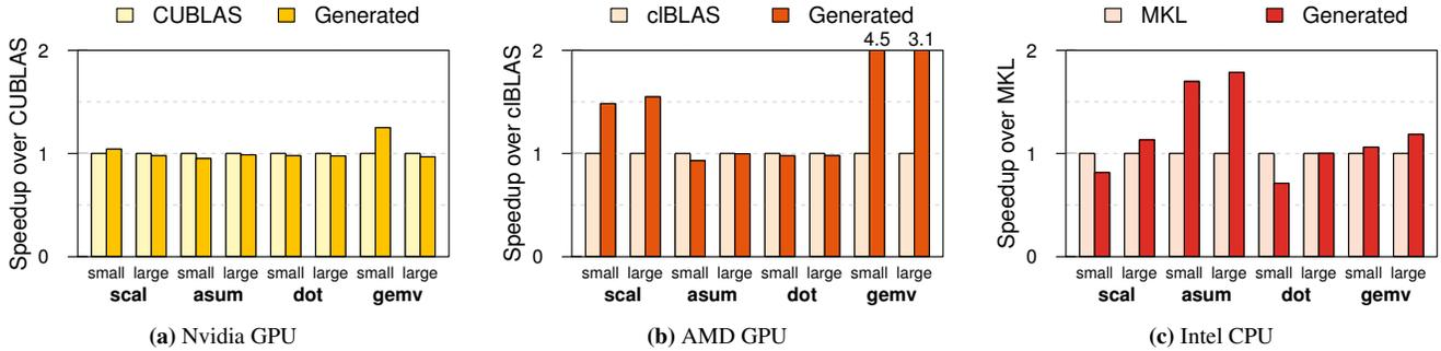
**Figure 11:** Performance comparison of our approach relative to a highly-tuned platform-specific library; CUBLAS for Nvidia, cBLAS for AMD and MKL for the CPU. Our approach matches the performance of CUBLAS and MKL, and outperforms cBLAS on some routines.
