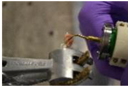
Fig. 5: Image of Novel Ultrasound Cutting Device driven by cymbal transducer.
