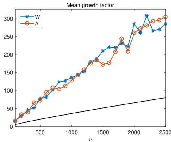
FIG. 3.1. Mean growth factors for partial pivoting on orthogonal matrices  $W$  from the Haar distribution and on  $A = W + xy^T$ , where  $x$  and  $y$  are generated with elements from the uniform distribution on  $[0, 1]$  and then scaled so that  $\|x\|_2 = \|y\|_2 = 1$ . The mean is over 12 matrices  $A$  and  $W$  for each  $n$ . The black curve is  $n/(4 \log n)$ .
