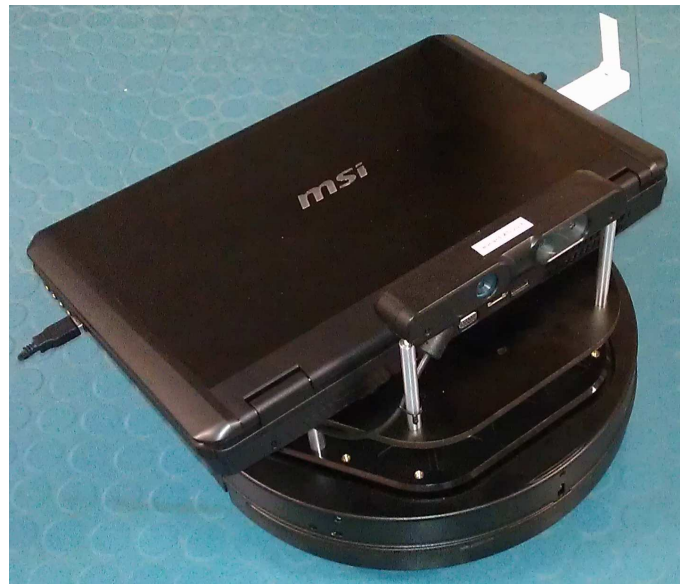
Fig. 1: Photograph of the Turtlebot 2 platform used in our experiment. It is a 2-wheeled platform with an RGB-D sensor, controlled by an onboard computer (a standard laptop in this scenario).
