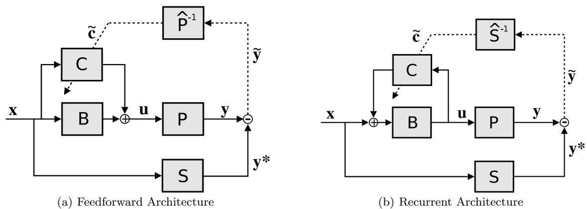
**Fig. 3** Schematic of feedforward and recurrent architectures
