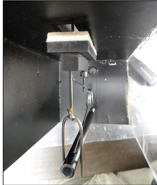
Fig 4. The felted and leathered pallet installed in the pallet box. The pallet is held open by the rod visible just above the middle of the front of the pallet and passing through the pallet opening.
