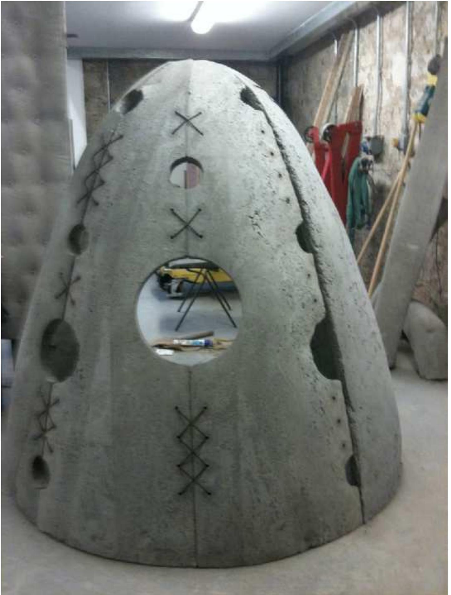
Figure 5: Interwoven geocomposite material
