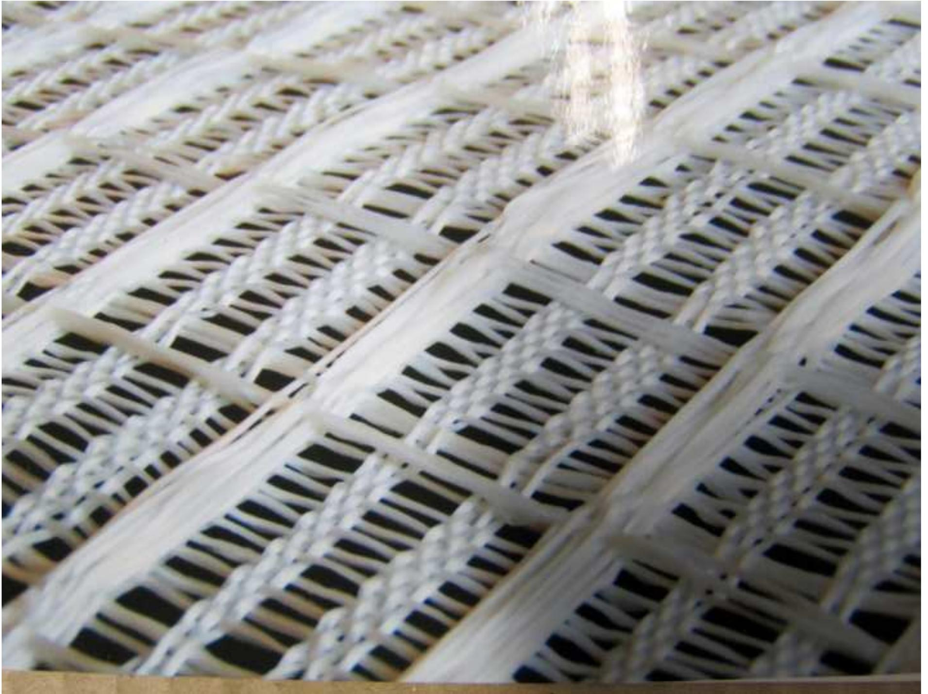
Figure 6: Manufacturing double layer fabric
