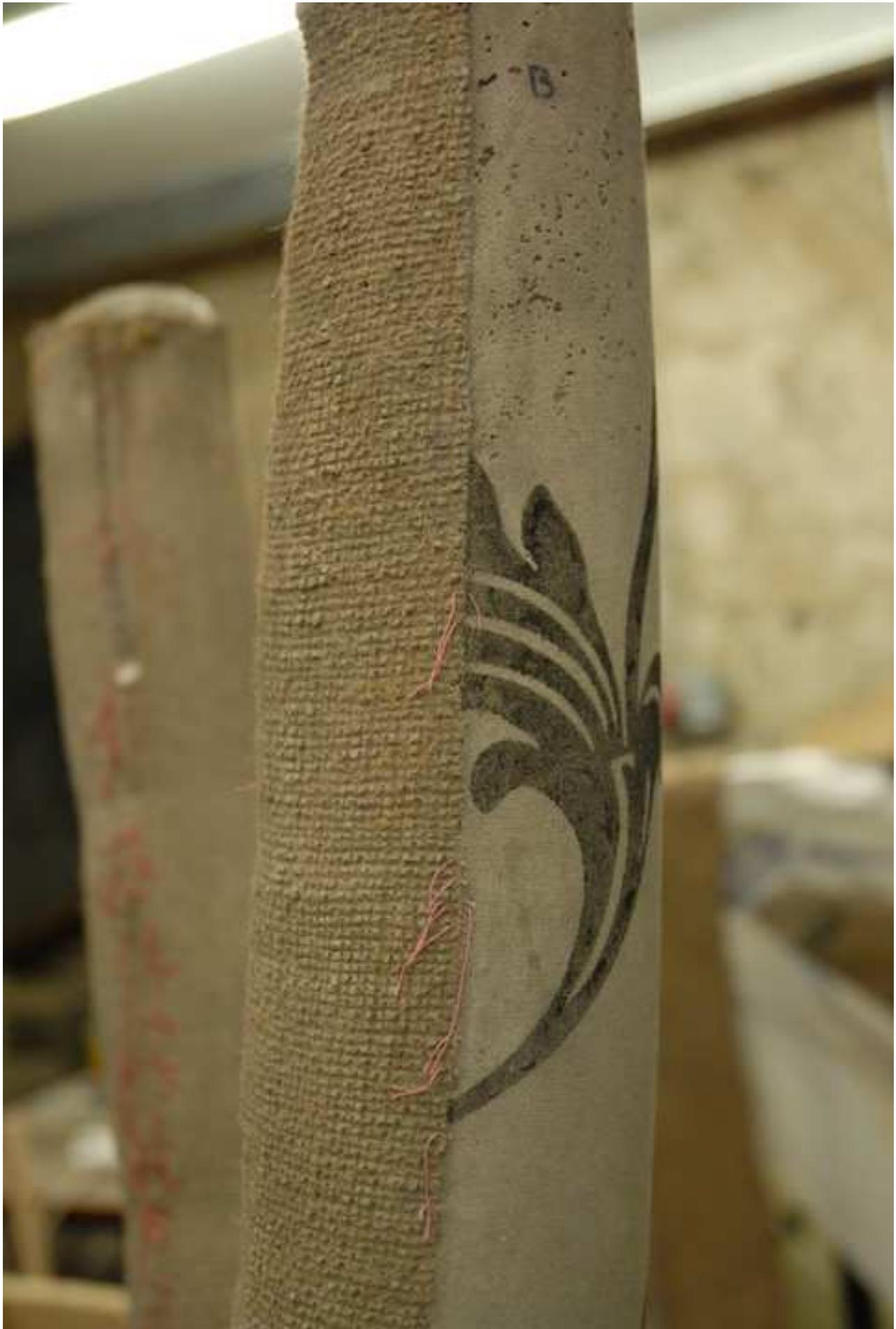
Figure 3: Formwork panels with range of surface finishes
