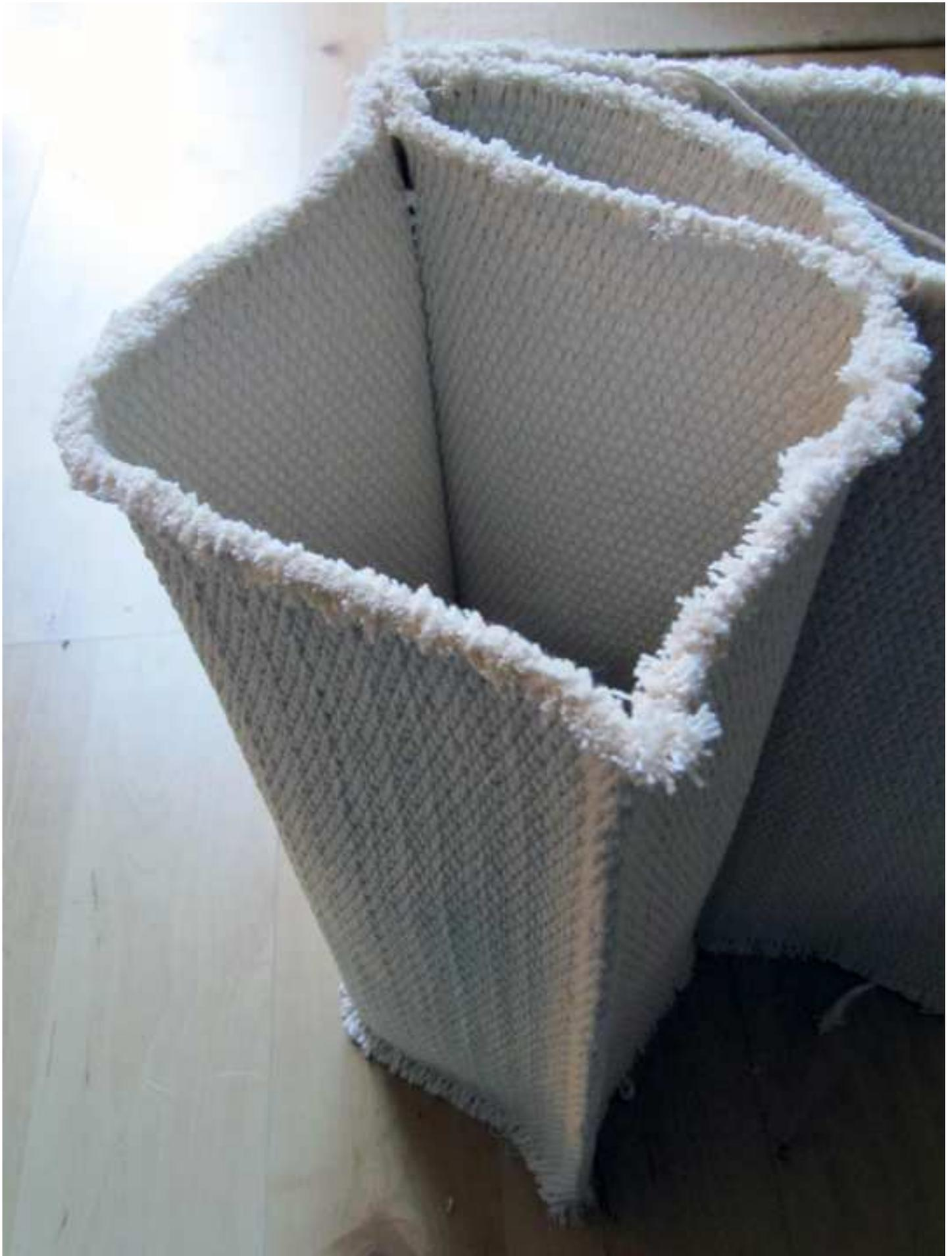
Figure 11: 3D tapered woven preform
