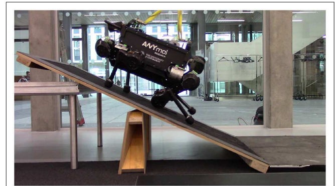
FIGURE 8 | ANYmal climbing up on a 30^\circ slope.
