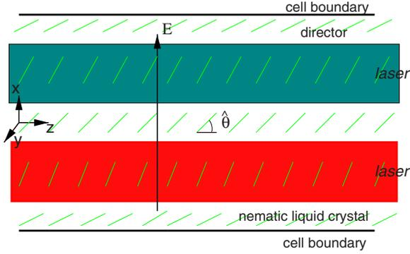
FIG. 1. (Color online) Schematic diagram of a liquid crystal cell with two polarized light beams of different colors.
