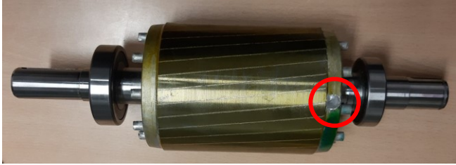
Fig. 10. The rotor with one broken rotor bar.
