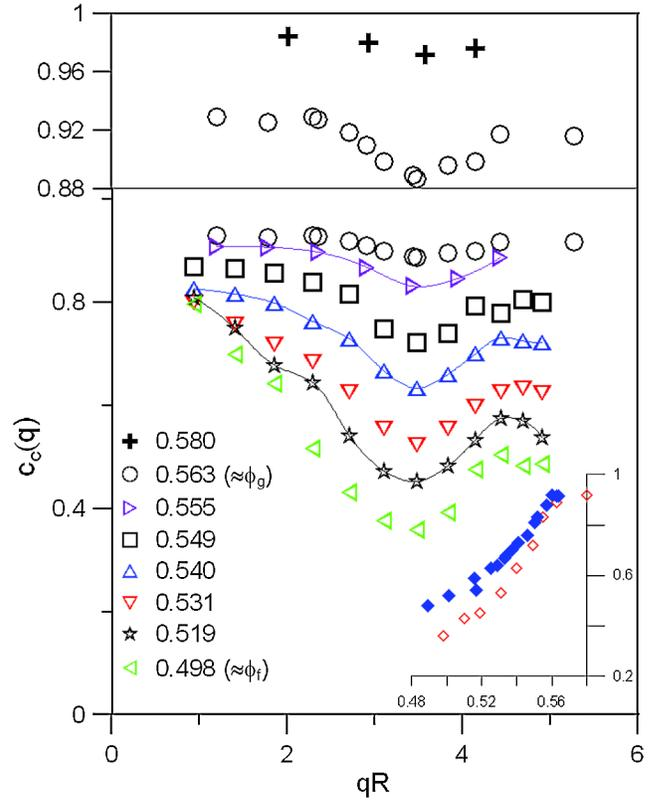
FIG. 2 (color online). Stretching indices [defined in Eq. (3)] versus wave vector for the volume fractions indicated. The scale of the top panel is 4 times that of the bottom panel. The data for  $\phi = 0.58$  are for an “aged” sample (see Ref. [18]). Lines drawn on alternate data sets are guides to the eye. The inset shows  $c_c(q_m)$  (open diamonds) and  $c_s$  (filled diamonds) for all experimental volume fractions.
