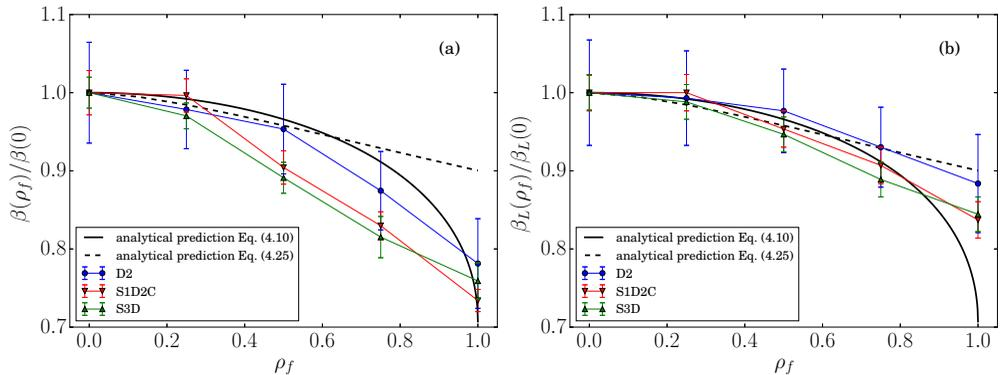
FIGURE 1. (Colour) Value of  $\beta$  as a function of  $\rho_f$  normalised by its value at  $\rho_f = 0$  from datasets D2, S3D and S1D2C compared to the analytical predictions in Eqs. (4.10) and (4.25). (a):  $\beta = \varepsilon L_f / U^3$ , (b):  $\beta_L = \varepsilon L / U^3$ , where  $L$  is the integral scale.
