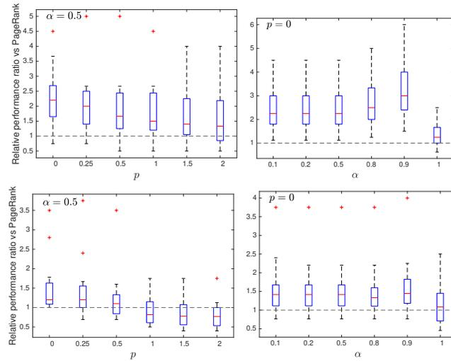
**Figure 9.** Link prediction performance comparison on two network dataset: UK FACULTY dataset (top) and SMALL WORLD CITATION network (bottom). The plots show means and quartiles of the ratio between the fraction of correctly predicted edges using  $S_{\mathcal{M}}$  and the one obtained using  $S_{PR}$ , over ten random trials for different values of  $p$  and  $\alpha$  in (3.2).
