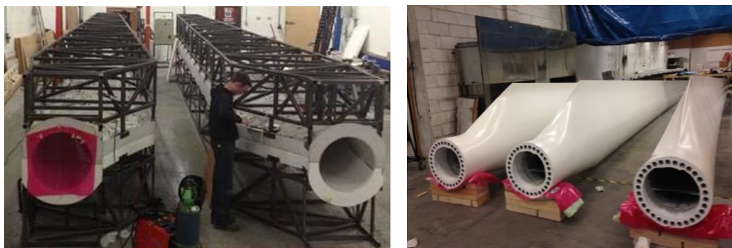
Figure 1: Integrally-heated ceramic moulds for manufacturing 12.6 m wind turbine blades (left), and the finished turbine blades made from glass-fibre/epoxy-powder (right).
