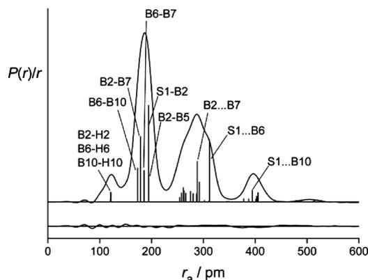
**Fig. 2** Experimental radial-distribution curve and theoretical-minus-experimental difference curve for the refinement of 1-SB<sub>9</sub>H<sub>9</sub>. Before Fourier inversion the data were multiplied by  $s \cdot \exp(-0.00002s^2) / (Z_s - f_s)(Z_B - f_B)$ .
