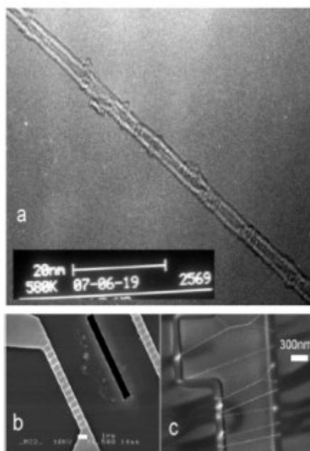
**Figure 3.** (a) TEM picture of SWNT crossing a slit in the growth substrate (200 kV, Philips CM200), (b) SEM picture of the substrate used for these studies, (c) SEM picture of SWNT grown across a slit, showing the tendency of the nanotubes to bundle as they cross.
