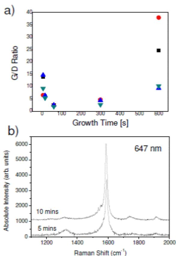
**Figure 5.** (a) Plot of the G/D ratio determined by fitting the spectra in (b) as a function of growth time. The different symbols represent measurements at different laser wavelengths (squares: 514 nm, circles: 568 nm, up-triangles: 647 nm, down-triangles: 785 nm). (b) Absolute intensity in the G–D region for 5 min and 10 min growth, using a laser excitation wavelength of 647 nm. The absolute intensity of the D-peak decreases as the growth time increases from 5 to 10 min.
