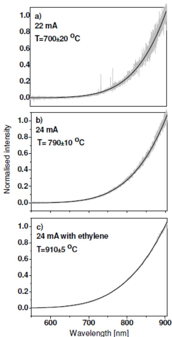
**Figure 2.** Blackbody radiation measurements to determine the temperature of the local heater. (a, b) Measurements made before the introduction of the hydrocarbon precursor for electrode currents of 22 mA and 24 mA, respectively. (c) Measurement made after introduction of ethylene for a current of 24 mA. The blackbody formula (see text) was fitted to the data yielding the temperatures given on the plots.
