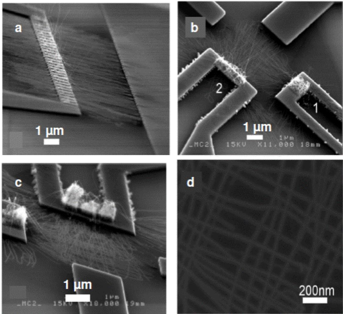
**Figure 1.** Examples of SWNT arrays grown from Mo electrodes using the local heating method (ethylene hydrocarbon precursor with Fe catalyst). The substrates were tilted by 20°. (a) SWNT aligned during growth in the presence of a DC electric field (1 V/lm) (b) and (c) sequential growth of SWNT arrays. In (c) small vertically aligned MWNT arrays were first grown as the electrode temperature was increased. (d) Magnification of crossed SWNT from (b).
