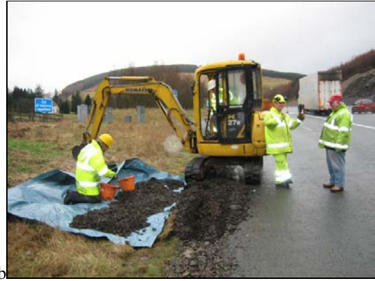
Figure 3. Soil water collection (a) and filter drain sediment sampling (b) at Basin 29A
