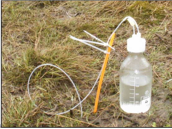
Figure 3. Soil water collection (a) and filter drain sediment sampling (b) at Basin 29A
