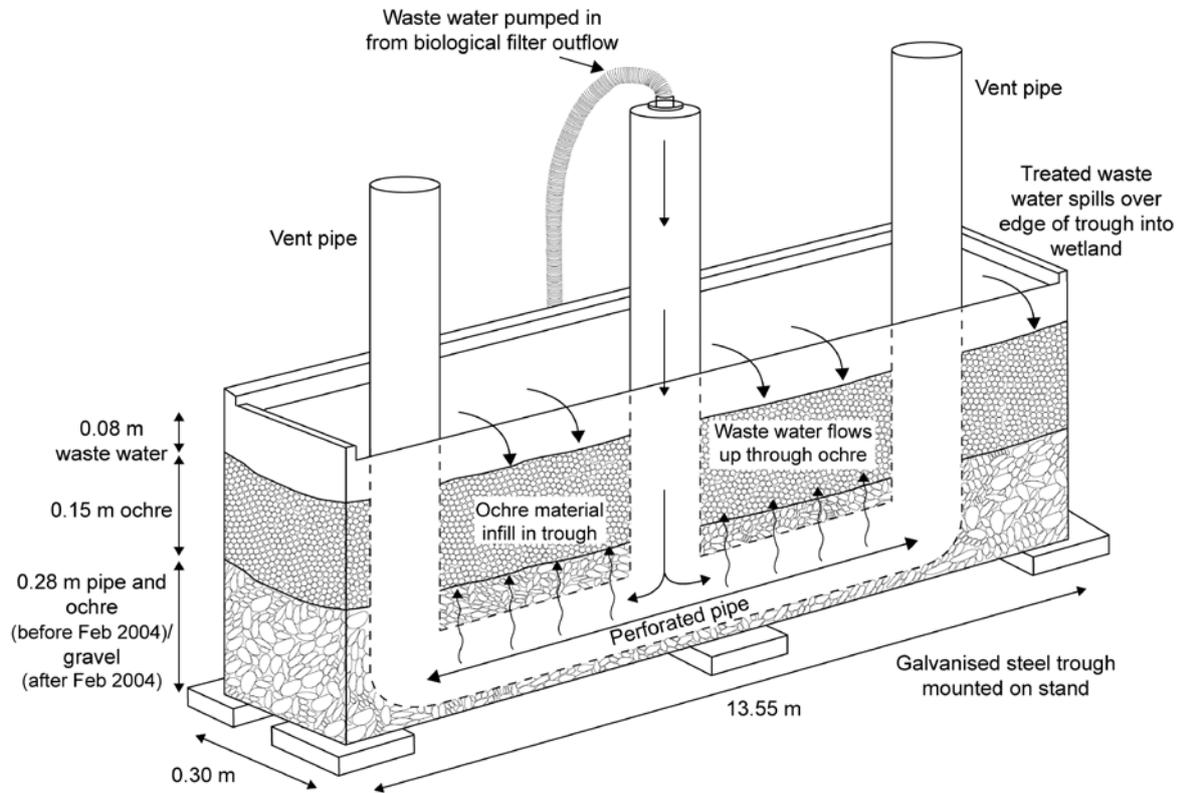
Figure 2. Schematic diagrams (not to scale) of the tank containing ochre pellets in the experiment to treat final effluent at Windlestone WWTP for (a) horizontal saturated flow conditions, and (b) vertical saturated flow conditions.
