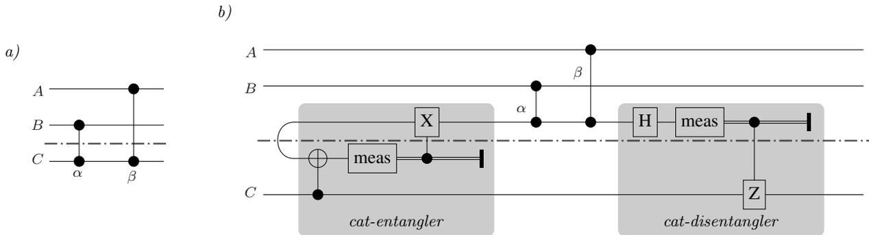
FIG. 2. Implementation, as in [30], of a group of nonlocal CZ gates that share a common qubit. Circuit *a*) is the original circuit, *b*) is the distributed version. The dashed line indicates how the circuit is separated into two QPUs. The bent wire on the left of *b*) represents an ebit. The measurement outcomes are communicated through a classical network.
