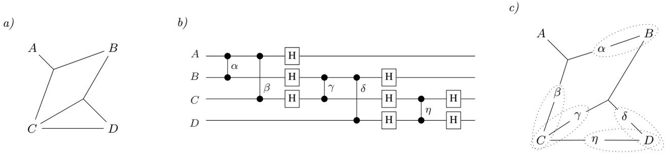
FIG. 10. *a)* An arbitrary input hypergraph. *b)* A (not unique) dummy circuit built from the hypergraph. *c)* The hypergraph obtained by applying the algorithm from Figure 4 on the dummy circuit, the hypergraph obtained is an extended version of the input one. We can retrieve the input hypergraph by merging vertices as indicated by the dotted ellipses.
