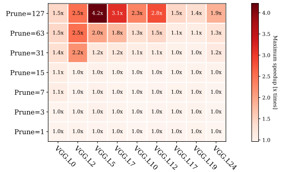
Fig. 16. Speedups observed when pruning at different distances within each layer of VGG-16 using the Arm Compute Library GEMM implementation.
