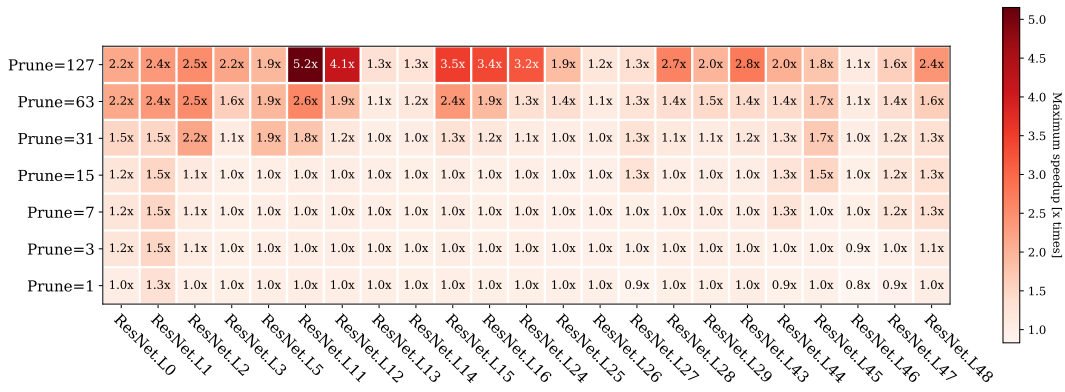
Fig. 13. Speedups observed when pruning at different distances within each layer of ResNet-50 using the Arm Compute Library GEMM implementation running on HiKey 970.
