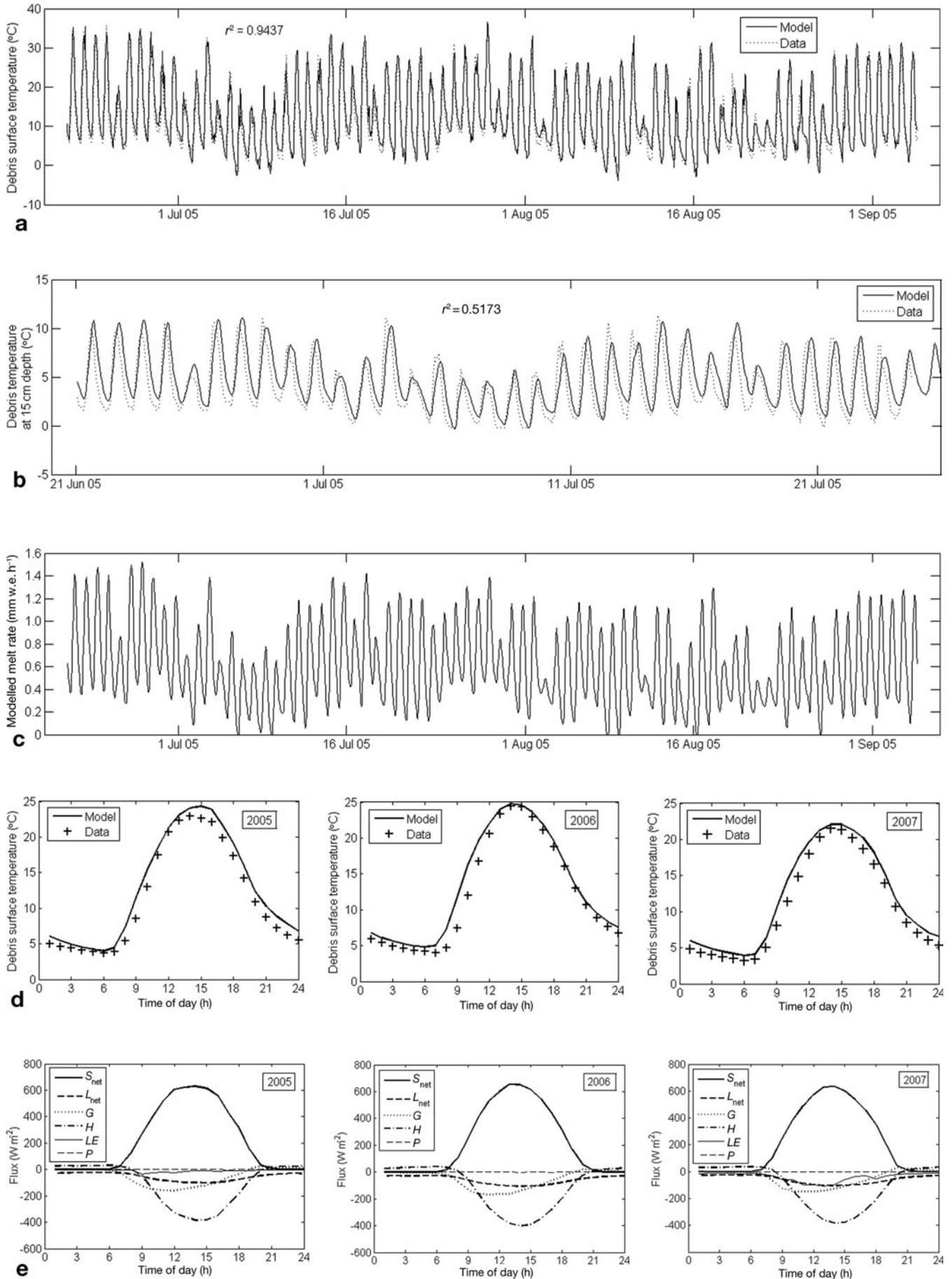
**Fig. 3.** Model outputs for the Miage glacier AWS site (2030 m a.s.l.) using the default parameter values listed in Table 1. (a) Modelled and measured debris surface temperature, (b) debris internal temperature at 15 cm depth and (c) modelled hourly melt rate for the 2005 ablation season. (d, e) Mean daily cycles of modelled and measured debris surface temperature (d) and surface heat fluxes (e), for the ablation seasons of 2005, 2006 and 2007.
