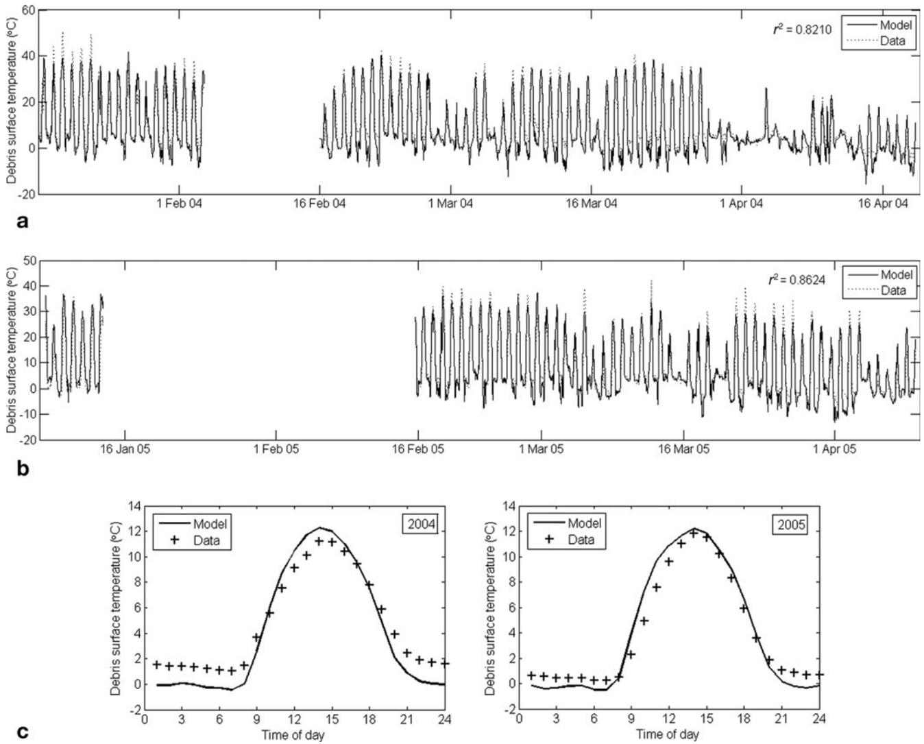
**Fig. 5.** Model outputs for Villarrica glacier using the default parameter values listed in Table 1. Modelled and measured debris surface temperature in (a) 2004 and (b) 2005, and mean daily cycles of surface temperature in (c) 2004 and (d) 2005.
