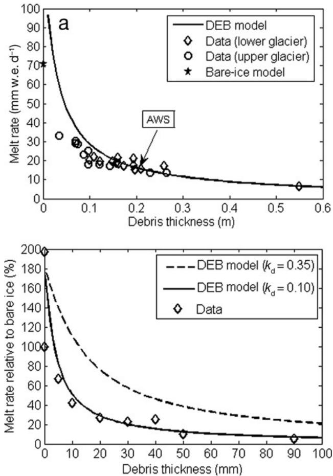
**Fig. 6.** Modelled and observed mean daily melt rates plotted against debris thickness, for (a) Miage glacier and (b) Villarrica glacier. Note that the data used to run the DEB model for Miage glacier (a) were recorded at an AWS (indicated data point) on the lower glacier. Melt data from the upper glacier, where meteorological conditions are quite different, are shown separately because they should not be directly compared to the curve.
