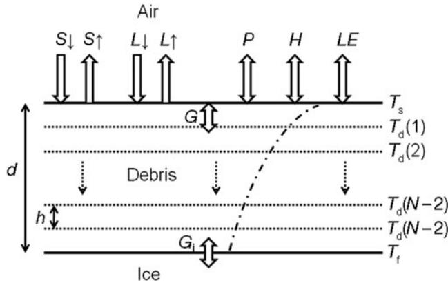
**Fig. 1.** Schematic of the DEB model showing heat fluxes at the top and bottom of a debris layer of thickness  $d$ . The debris temperature is calculated for  $N$  layers of thickness  $h$ , with boundary conditions defined by the surface temperature,  $T_s$ , and the temperature of the debris/ice interface, which is assumed to stay at  $T_i = 0^\circ\text{C}$ . The dash-dot curve is an example temperature profile, where temperature increases towards the right.
