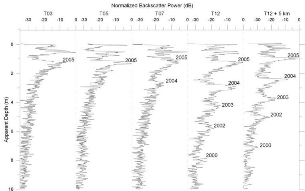
**Figure 3.** Normalized radar backscatter power return with depth across the percolation zone from T03 to T12, from measurements in April and May 2006. Centre frequency 13 GHz, bandwidth 8 GHz. Interpreted positions of summer melt surfaces are marked with dates. These surfaces correlate well with the surfaces tracked along EGIG from a borehole near summit using neutron probe density profiles.
