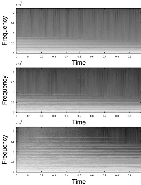
Figure 2: Spectrograms for synthetic struck plate sounds, under linear conditions (top), low velocity striking (middle) and high velocity striking (bottom).
