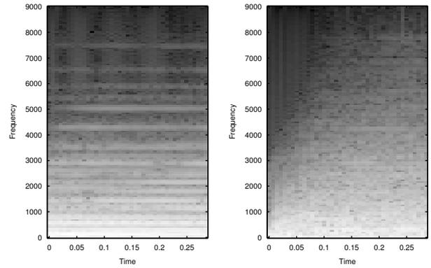
Figure 3: Spectrograms for initial segments of synthetic struck plate sounds, for small plate (left) and a large one (right).
