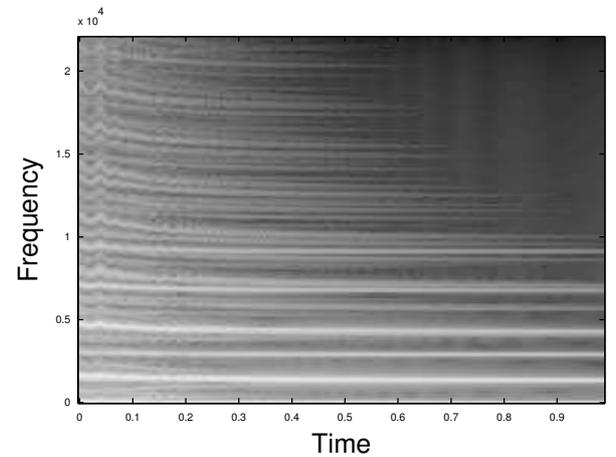
Figure 4: Spectrogram for a synthetic struck plate sound, showing initial wavering of partial frequencies, as well as downward glides.
