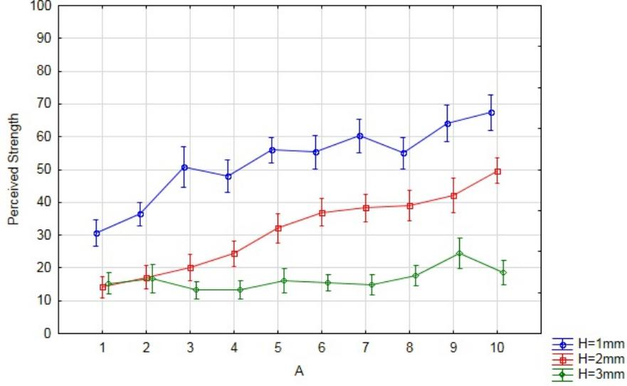
**Fig. 1.** Representation of responses for the perceived strength of the impact for all samples (percentage of cursor range). The level of the excitation  $A$  is presented on the horizontal axis, and each curve represents a level for the plate thickness. Dots denote the average value for all participants, vertical bars denote  $\pm$  standard errors.
