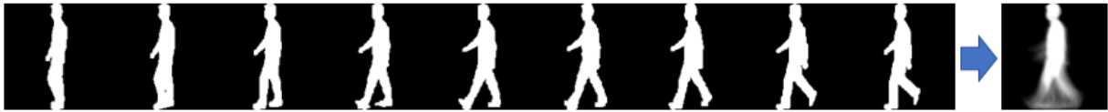
Figure 2: Gait energy image (image on right) is average of human silhouettes (images on left) in gait sequence.
