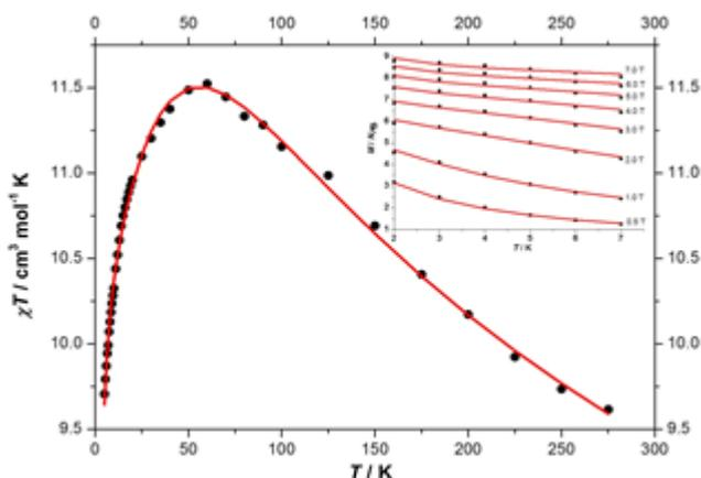
**Figure 13.** Plot of  $\chi_M T$  vs.  $T$  of **5**. Inset: Low temperature magnetisation vs. temperature (at various magnetic fields) plot of **5**. Solid red lines represent best fit to the experimental data.
