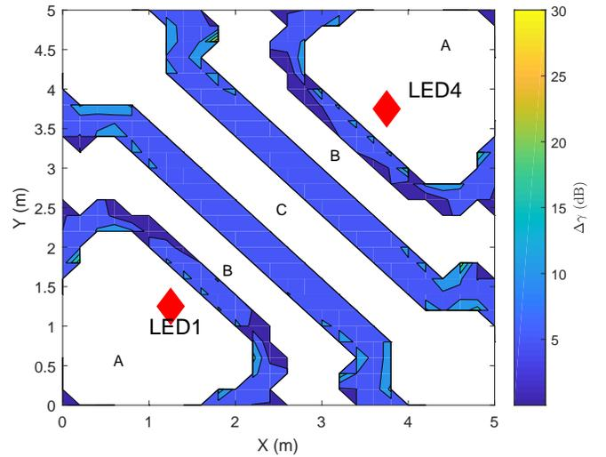
Fig. 13. The  $\gamma_b$  penalty incurred by S-CAP16 to achieve the FEC BER limit of  $3 \times 10^{-3}$  in an optical indoor multipath propagation with second-order reflections in comparison to LOS propagation. The white regions indicate region where  $\text{BER} > 3 \times 10^{-3}$ .
