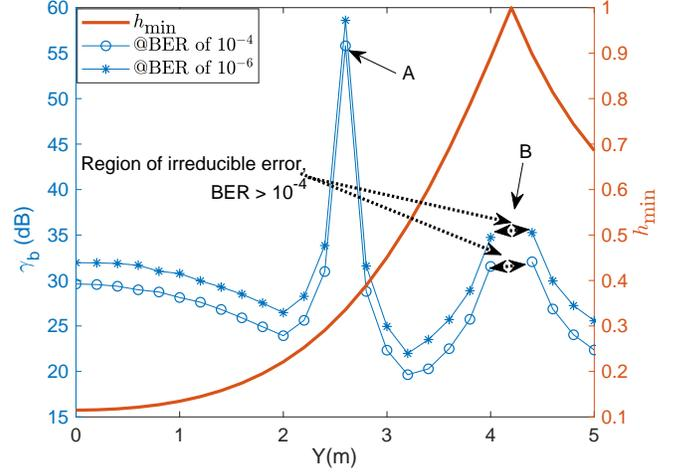
Fig. 9. SNR per bit penalty for S-CAP16 LOS propagation using LED1 and LED4 by considering a fixed location on x-axis ( $x = 0.8$  m) and varying the PD's location across the y-axis overlaid by the corresponding  $h_{\min}$  values.
