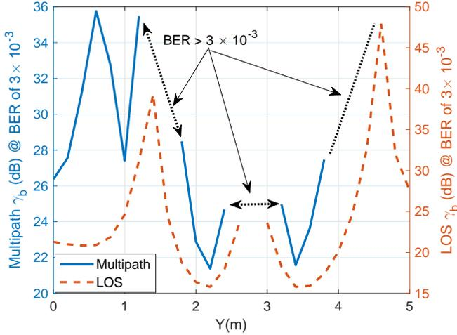
Fig. 14. Comparison of the BER performance trend of S-CAP16 in multipath and LOS propagation across the room for a fixed location on  $x$ -axis ( $x = 2.2$  m) and at the FEC BER limit of  $3 \times 10^{-3}$ .
