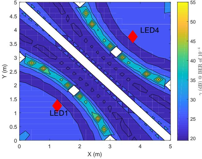
Fig. 7. The required  $\gamma_b$  for S-CAP16 LOS propagation to achieve BER of  $10^{-4}$  at each PD location across the room using LED1 and LED4 whose positions are shown by the red stars. The white region shows area of BER  $> 10^{-4}$ .
