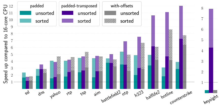
Fig. 8: Difference in GPU execution time speedup (when compared to a 16-core CPU) between the sorted and unsorted test suites, for each of the test layouts. The presented values are for the full test suite for each FSM. The FSM layout is dense .
