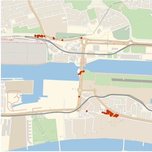
Figure 2: GPS location of a JCB 540-170 telehandler at the Connaught bridge Crossrail site in London between the 15th and the 19th of March 2016
