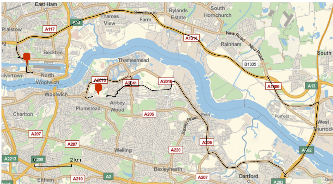
Figure 7: A bowser journey from the Connaught bridge site in North Woolwich to the Plumstead site of Crossrail on Tue, 21th of June; the bowser covered 47.6km in 1h and 31 minutes.
