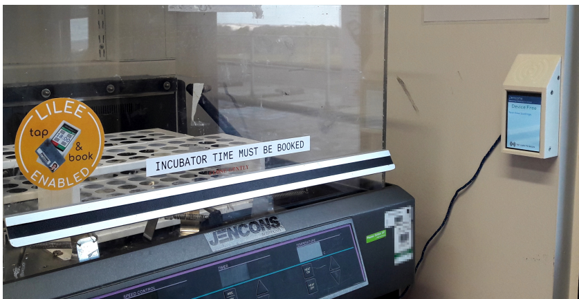
Fig. 10. A LILEE device wall-mounted alongside a shaking incubator.
