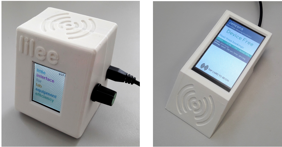
(a) Initial prototype with a small screen and rotary button on the side.
