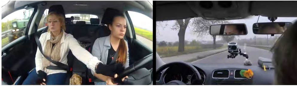
Fig. 26.1: Overtaken tractor is just passed, INS steers driving school's car back into lane
