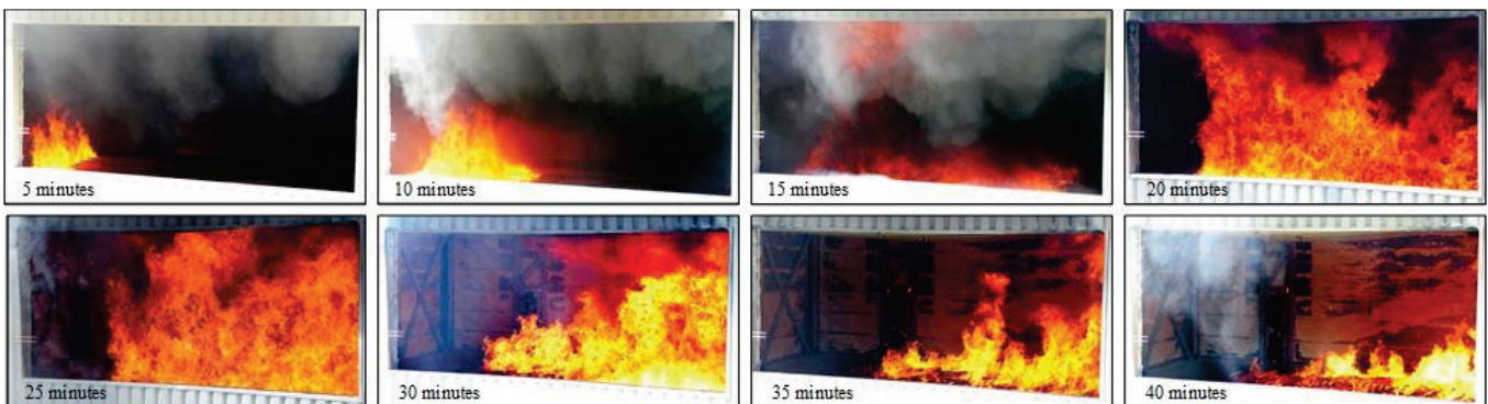
Fig. 4. Development of the fire during the test (photos provided by Horová K., CVUT in Prague).
