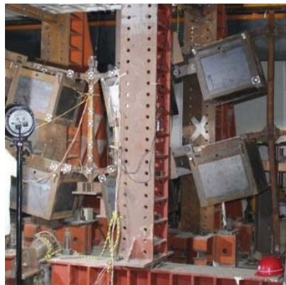
c. FRAME2 (middle and right photos show damages of columns)
