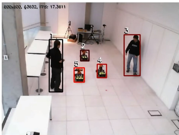
Fig. 1 Case study: multi-agent navigation system composed of autonomous robots (KUKA youBots), humans, and network cameras
