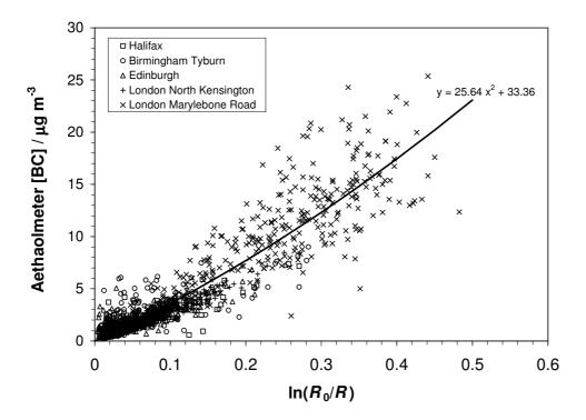
Figure 3: Linear fit to BC vs  $BSI_{BRITISH}$  for  $BSI_{BRITISH} < 15 \ \mu g \ m^{-3}$  at all sites.
