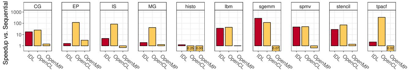
**Figure 19.** Speedup of our constraints based approach (executed on the best hardware and highlighted in red) compared to handwritten parallel OpenCL (executed on the GPU) and OpenMP (executed on the CPU) implementations.
