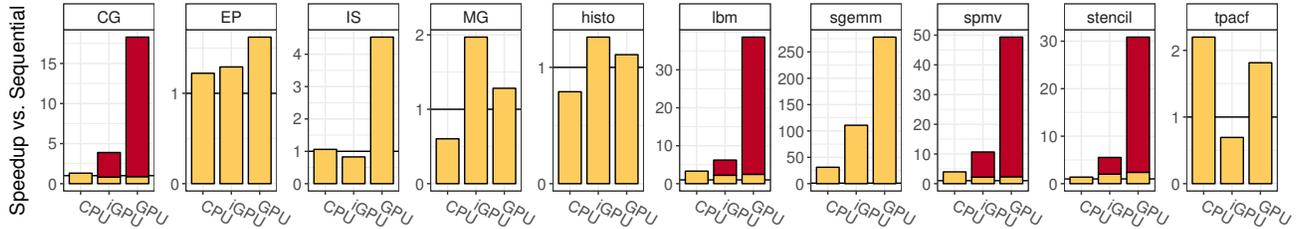
**Figure 18.** Speedup compared to the sequential C program. Results for the best performing heterogeneous API on each device are shown. The red bars indicate a manual runtime optimization for avoiding unnecessary data transfers.
