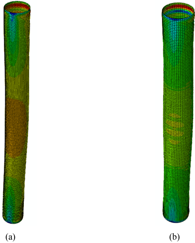
Figure 3: Finite element model of (a) specimen C2L2000 failed by flexural buckling, and (b) specimen C3L3000 failed by local buckling
