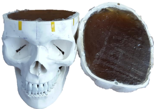
Fig. 7. Fabricated artificial head phantom
